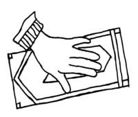
4. Inspect the seals. If there is no visible penetration of liquid throughout the sealing area within 5s, seals are considered as
